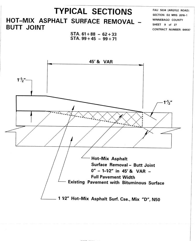
HOT-MIX ASPHALT APPLICATION RATES: All Hot-Mix Asphalt Mixtures: 112 lbs/sq.yd/inch Bituminous Materials (Prime Coat) = 0.05 LB/Sq. Ft.
