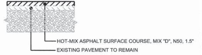
EXISTING PARKING LOT PAVEMENT OVERLAY
