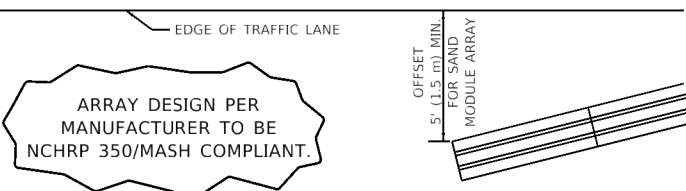
DETAIL "A" IMPACT ATTENUATOR, TEMPORARY (SEE NOTE 5)
