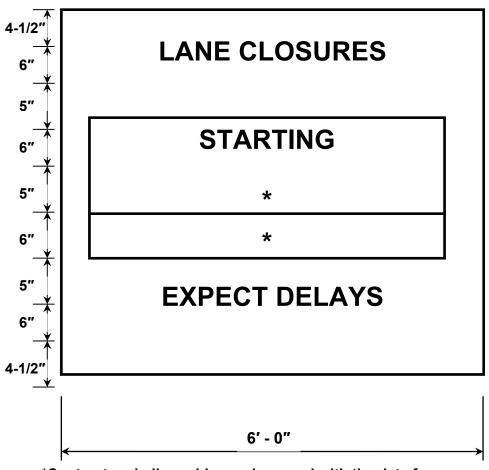
\*Contractor shall provide overlay panel with the date for Start of lane closure. Signs shall be erected a minimum of one (1) week in advance of the start of the work. Overlay panel shall be removed soon after start of construction.
