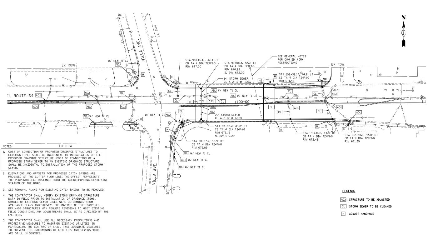
6. MANHOLES TO BE ADJUSTED SHALL BE ADJUSTED WITH A NEW TYPE 1 FRAME AND CLOSED LID AS NOTED ON THE PLANS. IF A MANHOLE ADJUSTMENT DOES NOT CALL OUT A PROPOSED FRAME AND LID, IT SHALL REUSE THE EXISTING FRAME AND LID.
