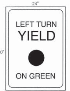
DETAIL A TRAFFIC SIGNS N.T.S. R10-12 MAST ARM MOUNTED 4 EACH REQUIRED SIGN PANEL - TYPE 1
