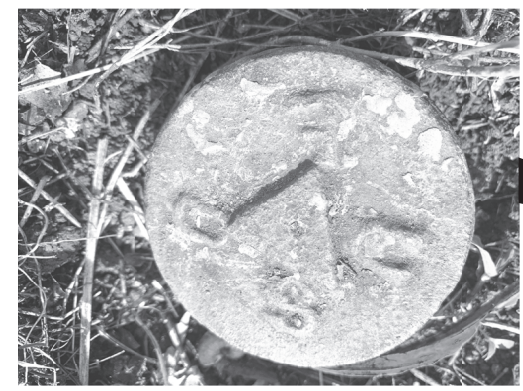
POC PARCEL 871926TE FOUND 3" STEEL PIPE W/ 3" STEEL CAP (APPARENT GOVERNMENT PROPERTY MARKER) POINT NO 283
