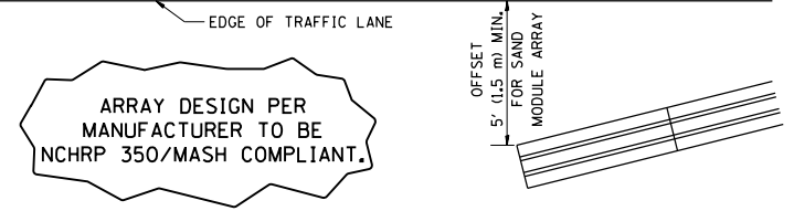
DETAIL "A" IMPACT ATTENUATOR, TEMPORARY (SEE NOTE 5)
