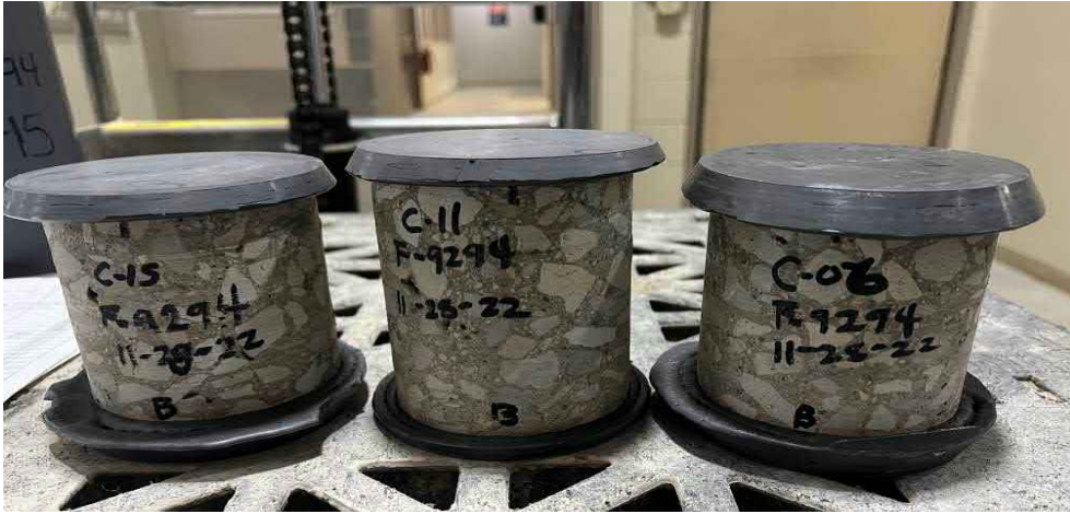
C-06, C-11, and C-15 concrete prior to testing.
