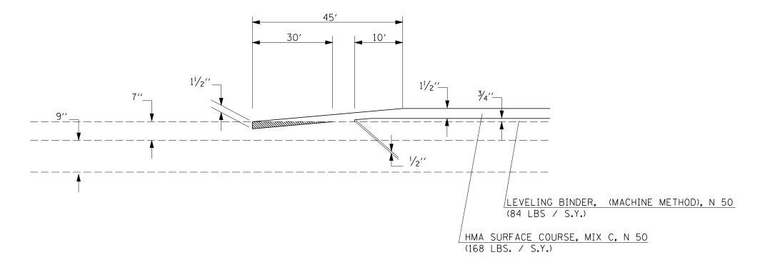
ILLINOIS DEPARTMENT OF TRANSPORTATION DETAIL OF HMA SURFACE REMOVAL - BUTT JOINT & TRANSITION SCALE: VERT.
