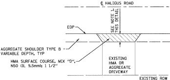
NOTES: 1. 5' MIN WHEN MATCHING EXISTING HMA DRIVEWAY 2' MIN. WHEN MATCHING EXISTING AGGREGATE DRIVEWAY
