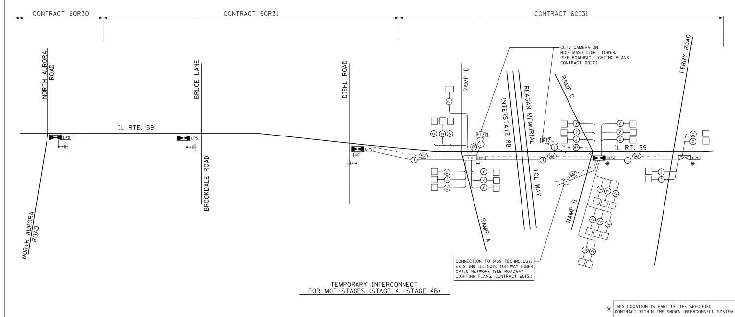
PERMANENT FIBER OPTIC CABLE SHALL BE IN PLACE BETWEEN THE DDI-COMMUNICATIONS CABINET AND FERRY ROAD, AND A TEMPORARY FIBER OPTIC CONNECTION SHALL BE IN PLACE IS BETWEEN THE DDI-COMMUNICATIONS CABINET AND DIEHL ROAD FOR ALL STAGES AFTER 3C.
