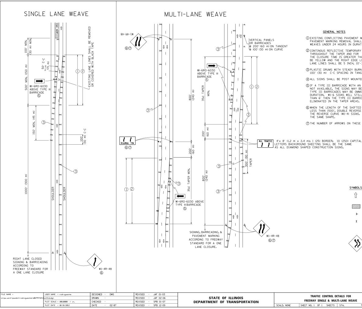
① EXISTING CONFLICTING PAVEMENT MARKING LINES SHALL BE REMOVED. PAVEMENT MARKING REMOVAL SHALL NOT BE REQUIRED FOR SINGLE LANE WEAVES UNDER 24 HOURS IN DURATION.
