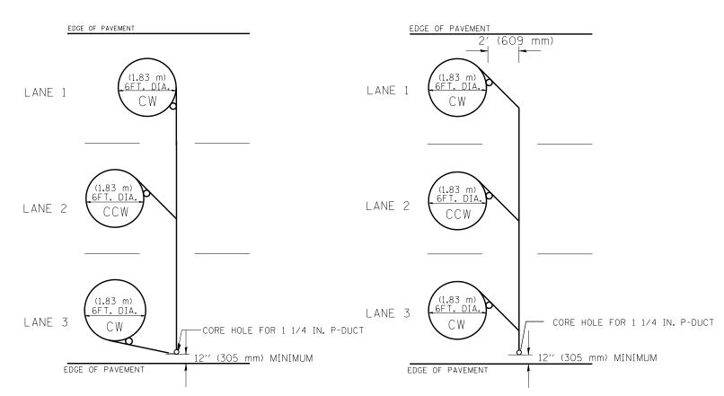
TYPICAL 6FT. (1.83 m) DIA. INDUCTION LOOP CORE DRILL
