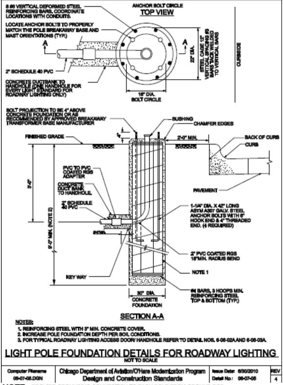
PROVIDE GROUNDING CONNECTION TO EACH POLE FROM GROUND ROD OF NEAREST HANDHOLE WITH #8 AWG BARE COPPER CONDUCTOR. THIS WORK IS INCIDENTAL TO PAY ITEM "LIGHT POLE CONCRETE FOUNDATION" AND NO EXTRA PAYMENT WILL BE MADE FOR THIS.
