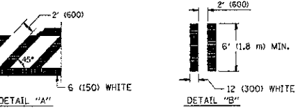
TYPICAL CROSSWALK MARKING
