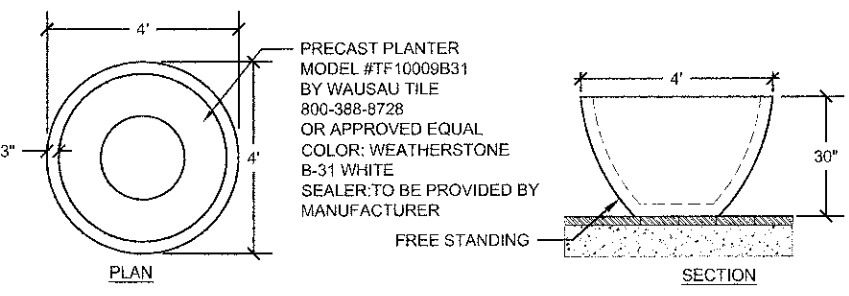
3 30" HT PRECAST CONC. PLANTER (QTY: 9) SCALE= 1/2"=1'-0"
