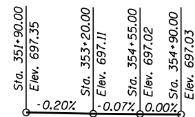
BNSF WEST BOUND TRACK PROFILE GRADE (Top of rail along South rail)
