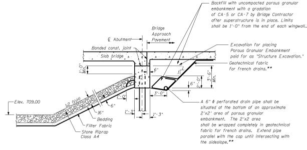
SECTION THRU INTEGRAL ABUTMENT
