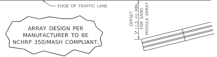
DETAIL "A" IMPACT ATTENUATOR, TEMPORARY (SEE NOTE 5)
