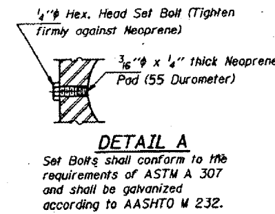
EXTERIOR NUT DETAIL (432 Required)
