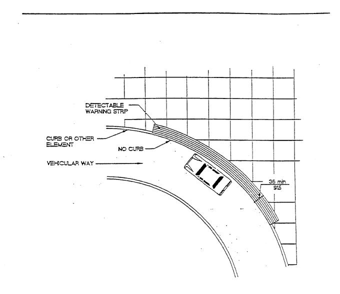
Fig 42 Detectable Warning at Hazardous Vehicular Areas 148
