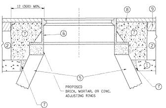
EXISTING BROKEN FRAMES AND LIDS SHALL BE REMOVED AND DISPOSED OF BY THE CONTRACTOR AND SHALL BE REPLACED AS DIRECTED BY THE ENGINEER. REPLACEMENT FRAMES AND LIDS WILL BE PAID FOR IN ACCORDANCE WITH ARTICLE 109.04 OF THE STANDARD SPECIFICATIONS UNLESS A SEPARATE PAY ITEM HAS BEEN PROVIDED.
