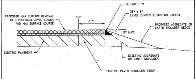
MILLING: WITH ADJACENT SHOULDER FLUSH WITH OR HIGHER THAN MILLED SURFACE
