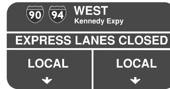
ELECTRONIC OVERHEAD SIGN TO DISPLAY "CLOSED" MESSAGE
