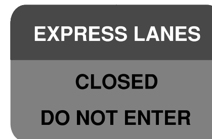
ELECTRONIC OVERHEAD SIGN TO DISPLAY "CLOSED" MESSAGE
