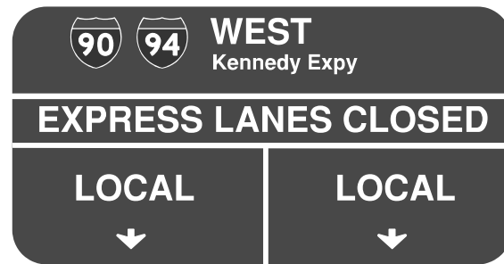
ELECTRONIC OVERHEAD SIGN TO DISPLAY "CLOSED" MESSAGE
