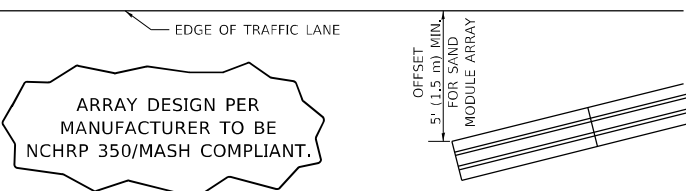
DETAIL "A" IMPACT ATTENUATOR, TEMPORARY (SEE NOTE 5)
