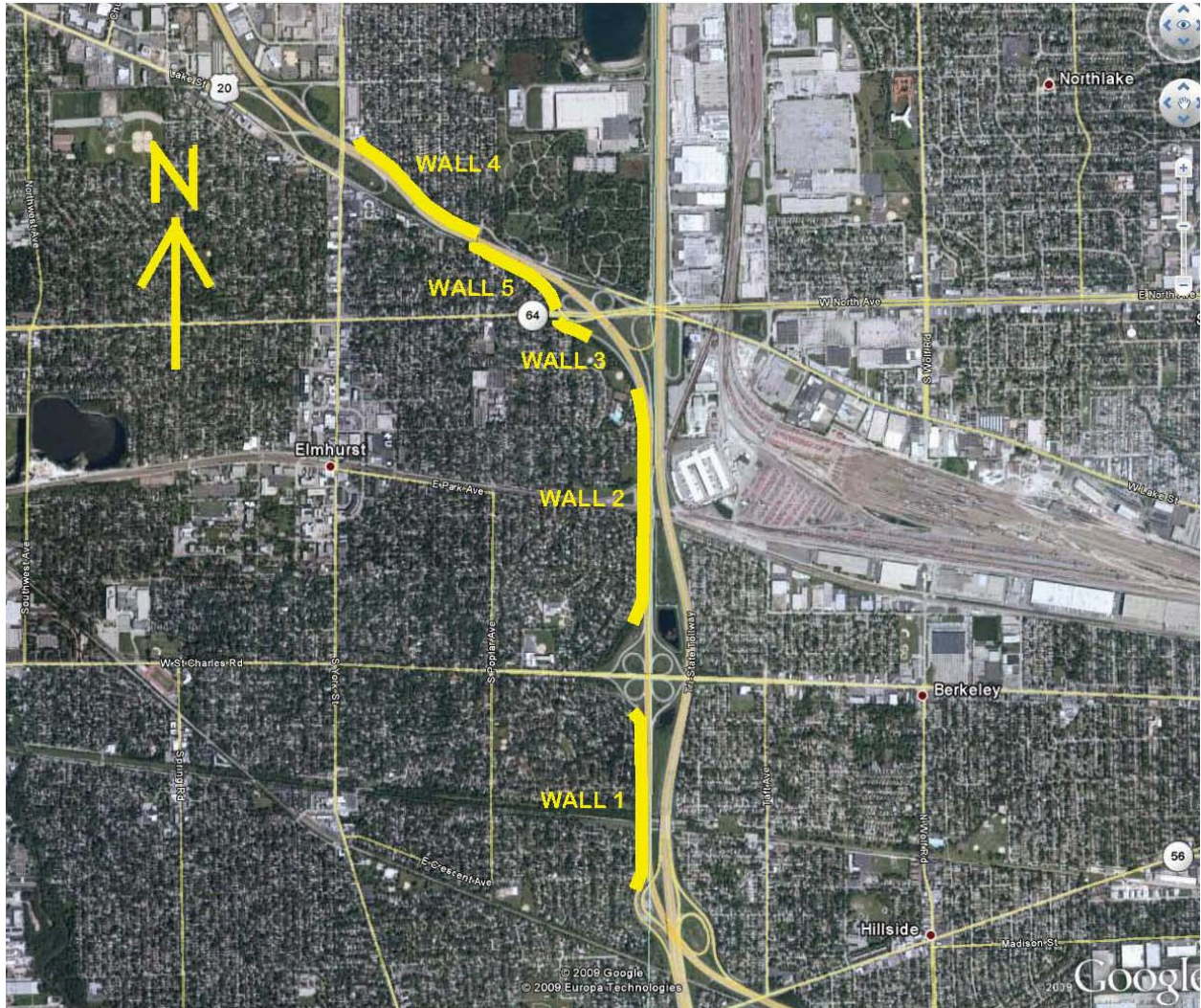
Figure 3. Noise Abatement Wall Locations
