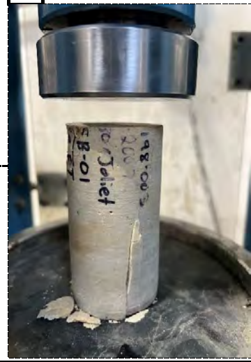
Type 3 Columnar vertical cracking through both ends, no well- formed cones
