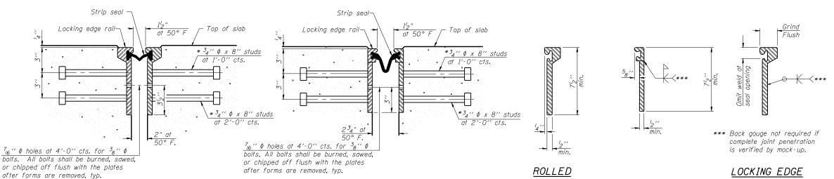
SECTION THRU ROLLED RAIL JOINT
