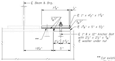
\*\* Cut existing anchor bolt flush with top of existing bearing plate. Cost included with Anchor Bolts, 1"
