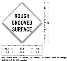
36.0" across sides 2.2" Radius, 0.8" Border, 0.6" Indent, Bi [ROUGH] C 2K 81% spacing; [GROOVED] C 2K 91% spacing; [SURFACE] C 2K 85% spacing;
