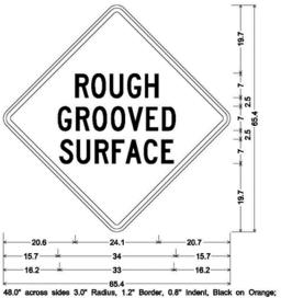
48.0" across sides 3.0" Radius, 1.2" Border, 0.8" Indent, Black on Orange; [ROUGH] C 2K 82% spacing; [GROOVED] C 2K 90% spacing; [SURFACE] C 2K 87% spacing;
