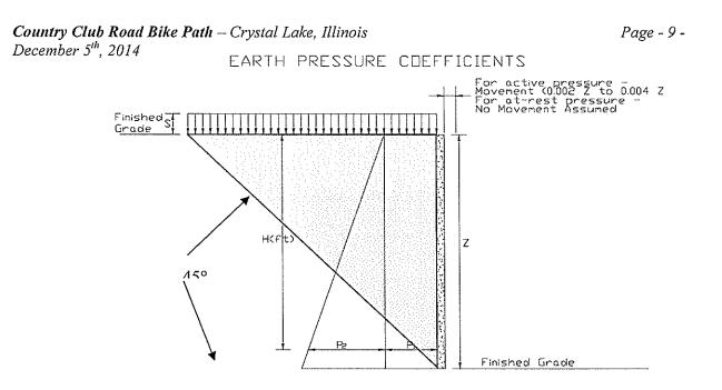
Lateral earth pressure is developed from the soils present within a wedge formed by the vertical below-grade wall and an imaginary line extending up and away from the bottom of the wall at an approximate 45° angle.
