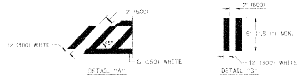
TYPICAL CROSSWALK MARKING
