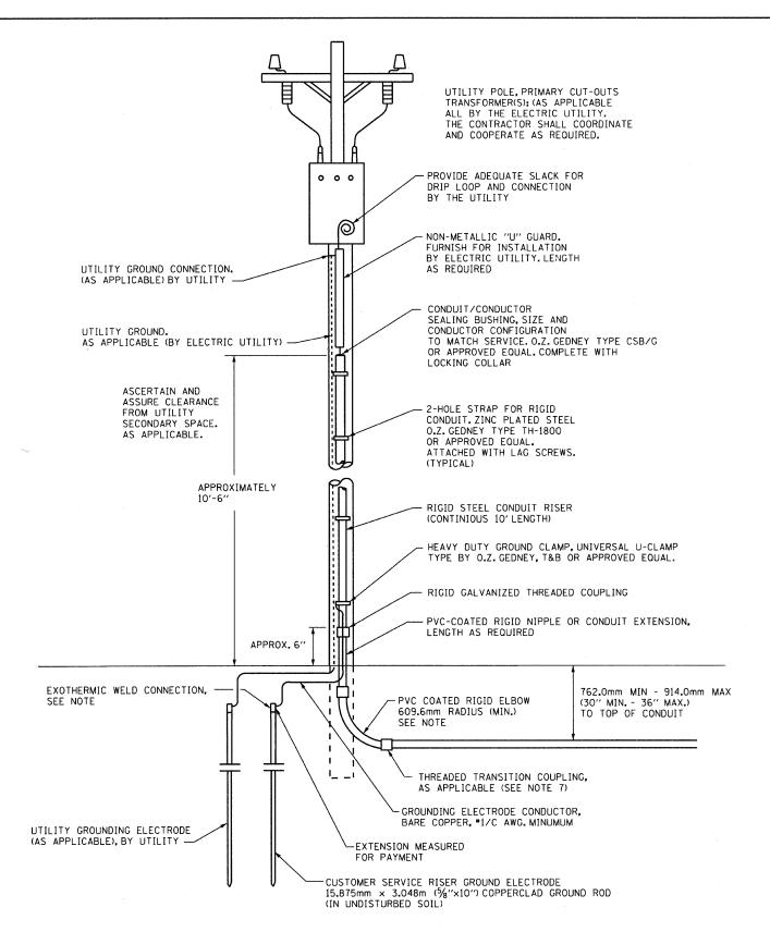
PROPOSED SERVICE INSTALLATION POLE TOP MOUNTED TRANSFORMER
