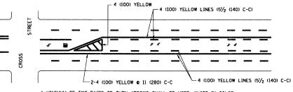
A MINIMUM OF TWO PAIRS OF TURN ARROWS SHALL BE USED, WHITE IN COLOR, ADDITIONAL PAIRS SHALL BE PLACED AT 200' (60 m) TO 300' (90 m) INTERVALS.
