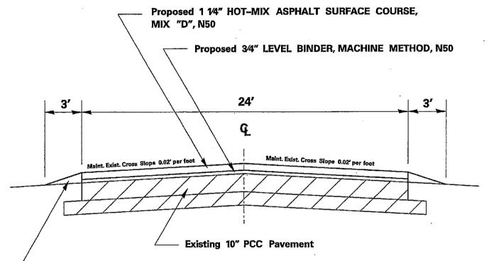
Proposed AGGREGATE WEDGE SHOULDER, TYPE B (Typical)
