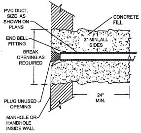
DUCT ENTRY DETAIL AT MANHOLES AND HANDHOLES
