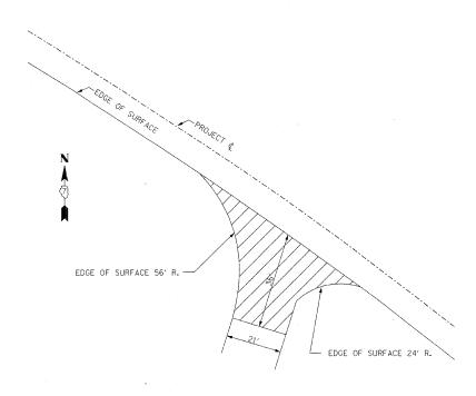
NOTE: THE SIDEROAD ABOVE SHALL HAVE A-2 BITUMINOUS SURFACE TREATMENT ON A PROPOSED 9" SOIL-CEMENT BASE IN THE AREA SHOWN.
