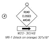
Post mounted sign with Type A Flashing Light
