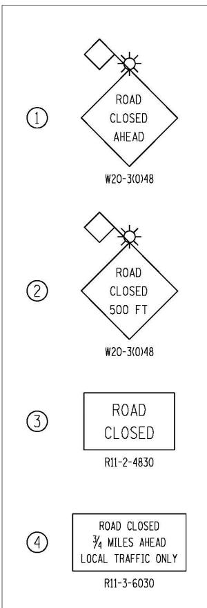
Post mounted sign with 18" x 18" (Minimum) orange flag and Type A Flashing Light.
