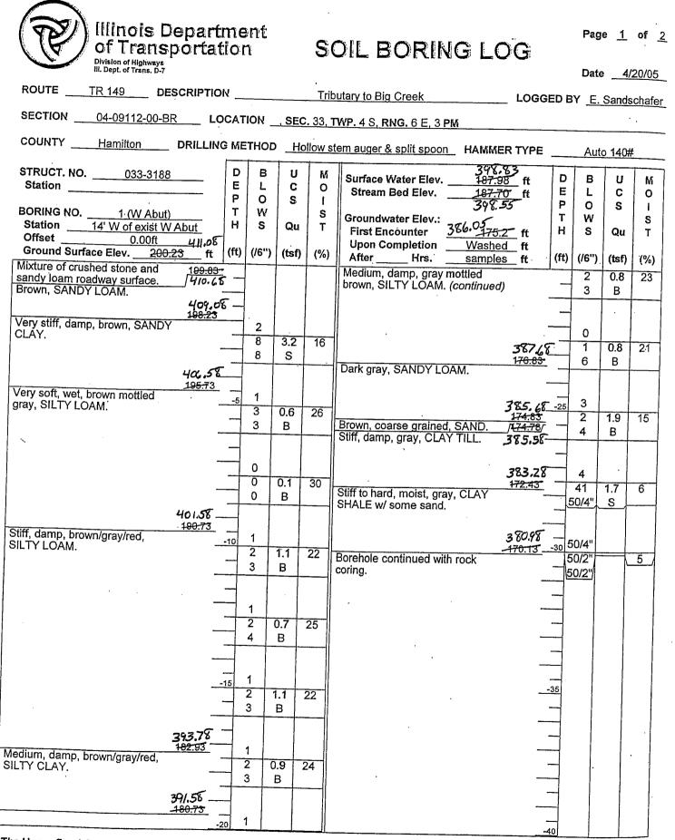
The Unconfined Compressive Strength (UCS) Failure Mode is indicated by (B-Bulge, S-Shear, P-Penetrometer) The SPT (N value) is the sum of the last two blow values in each sampling zone (AASHTO T206)
