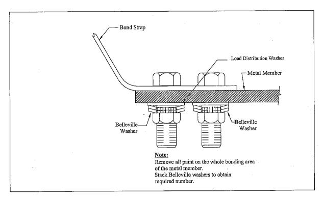
Figure I. Order of Assembly for Bolted Connections
