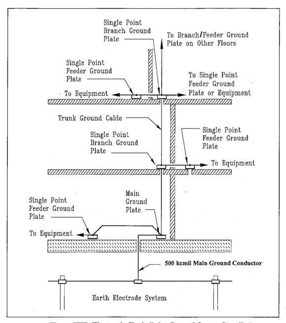
Figure XIII. Electronic Single Point Ground System Installation
