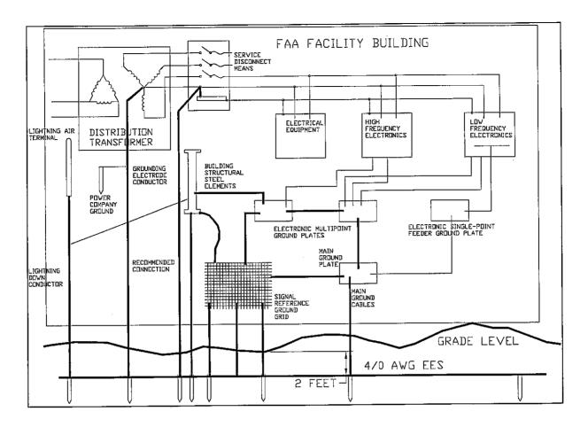
Figure XI. Facility Grounding System
