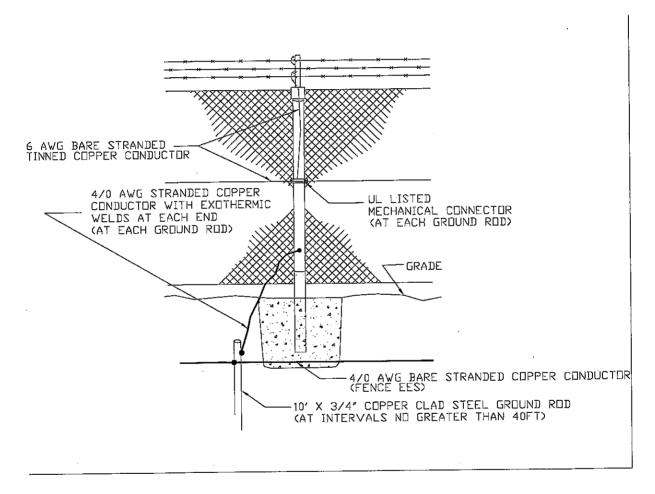
Figure VIII. Grounding Fences Requiring an EES
