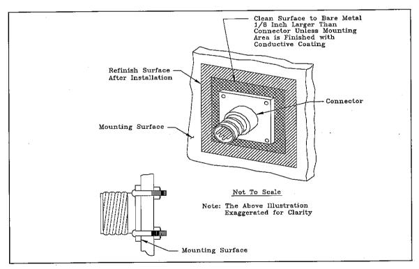
Figure II. Bonding of Connectors to Mounting Surface
