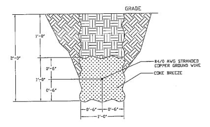
Figure IX. Grounding Trench Detail
