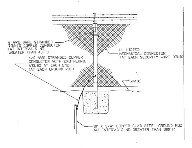
Figure VII. Fence Grounding
