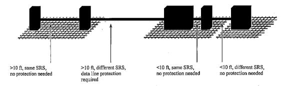
Figure XVI. Lines and Cables Requiring Protection
