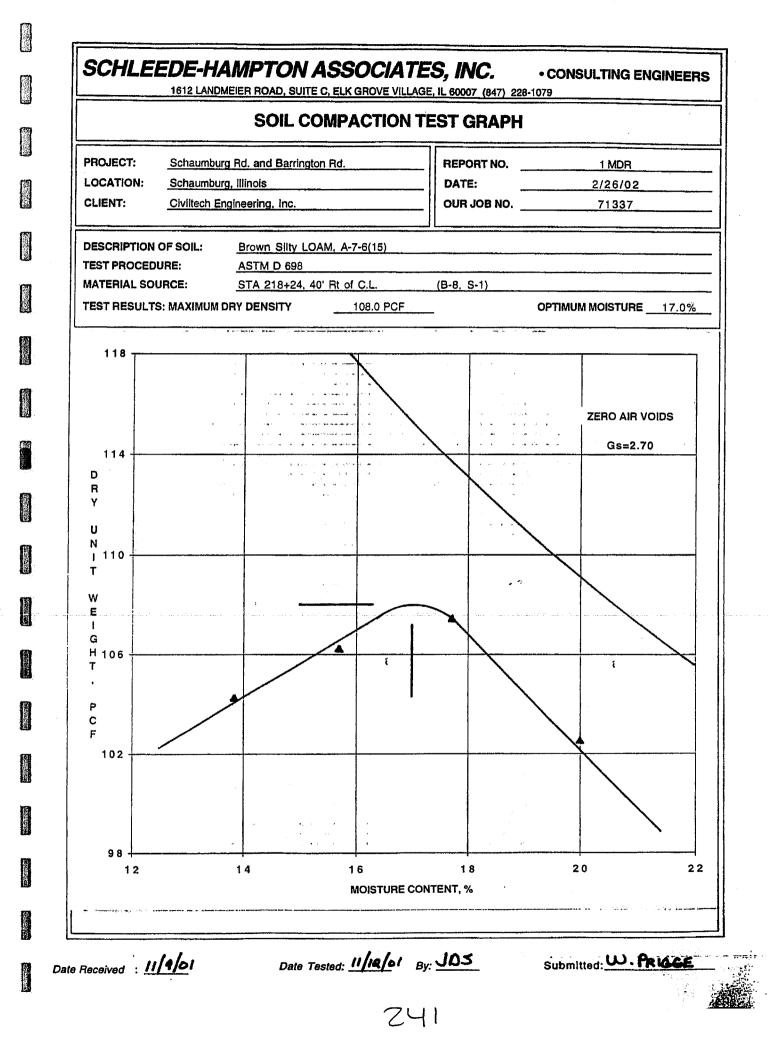
FILE NO .: 71337 Schaumburg Road and Barrington Road **PROJECT NAME:** SAMPLE I.D.: B-8, S-1 Brown and black Silty LOAM, A-7-6(15) **CLASSIFICATION:** MAX.UNIT WT.: 108.0 P.C.F. OPT. M.C.: 17.0 % **TEST UNIT WT.:** 104.2 P.C.F. TEST INIT. M.C.: 19.4 % TEST% of MAX. 96.5 %
