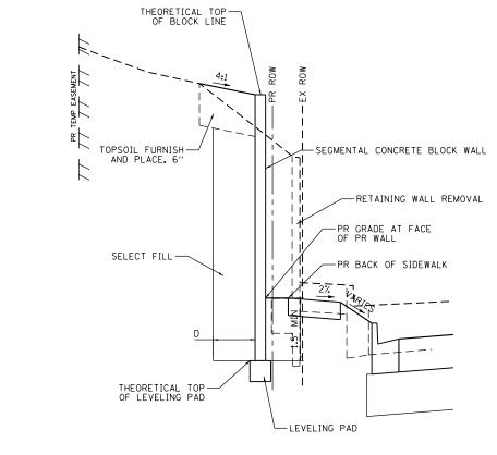
SEGMENTAL CONCRETE BLOCK WALL TYPICAL (IL 2)
