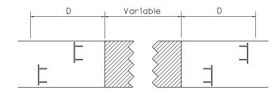
Type III Barricades and R11-4-4830 signs shall be as shown in "Road Closed To Thru Traffic" detail on Highway Standard 701901. If the distance "D" exceeds 2000' an additional set of barricades and R11-4-4830 shall be placed at each end of the work area.
