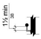
Circular Cross Section. Handrail gripping surfaces with a circular cross section shall have an outside diameter of 1½ inches minimum and 2 inches maximum.
