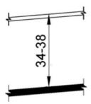
Clearance between handrail gripping surfaces and adjacent surfaces shall be 1½ inches (38 mm) minimum.
