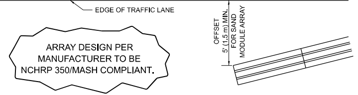
DETAIL "A" IMPACT ATTENUATOR, TEMPORARY (SEE NOTE 5)
