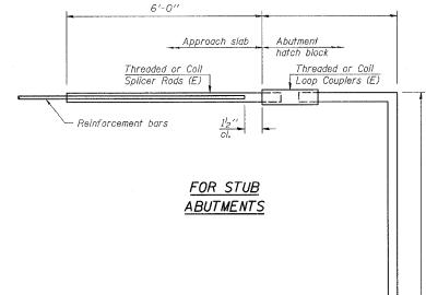
Bar Splicer for #5 bar Min. Capacity = 23.0 kips - tension Min. Pull-out Strength = 12.3 kips - tension No. Required =
