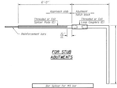
Min. Capacity = 23.0 kips - tension Min. Pull-out Strength = 12.3 kips - tension No. Required =
