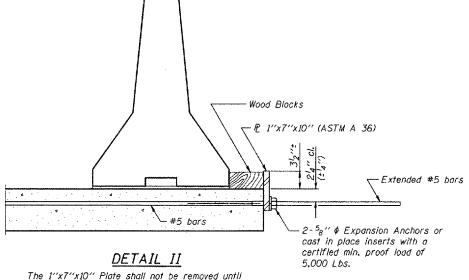
Stage II Construction forms and all reinforcement bars are in place and the concrete is ready to be
